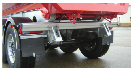
Hydraulic bumper controlled by the tipping mechanism
