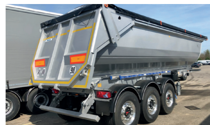
Hydraulic or mechanical angled topped reargate
