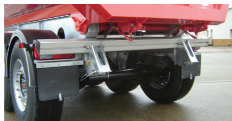
Hydraulic bumper controlled by the tipping mechanism
