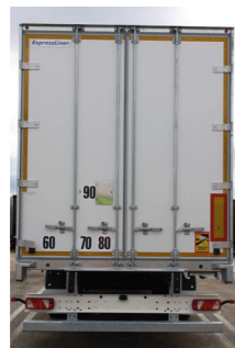
Double reardoor with 2 lockrods on the exterior of each doorleaf
