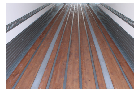
35 mm hardwood laminated flooring with steel omega profiles.
