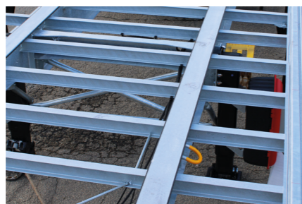
Mechanically welded platform with I-beams spaced at 400 mm intervals.
