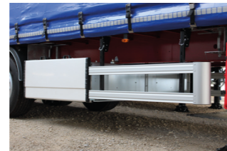
8 pallets in the wheelbase
