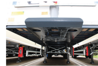
Reinforced coupling running plate
