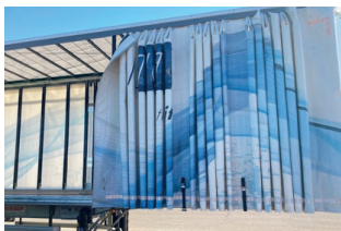
Tarpaulin folds completely in front, at the rear and in the centre
