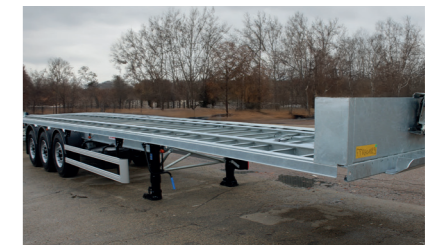
Hot dip galvanized chassis
