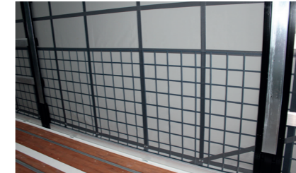
Reinforced anti-theft tarpaulin with reinforced stanchions
