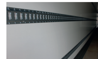
Cargo control tracks
