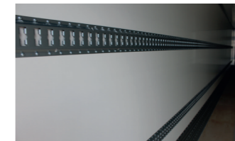
Cargo control tracks
