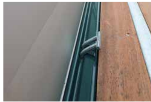
2.5-tonne lashing rings
