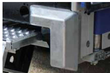
Full protection of the rear assembly with galvanized steel buffers
