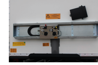
Side sliding system of couplings
