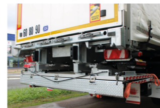
Retractable taillift DHOLLANDIA. Different lift capacity.
