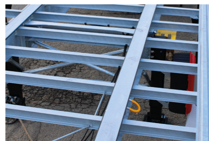
Mechanically welded platform with crossbeams in I spaced at 400 mm intervals.
