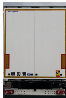
Double rear door with integrate lockrods
