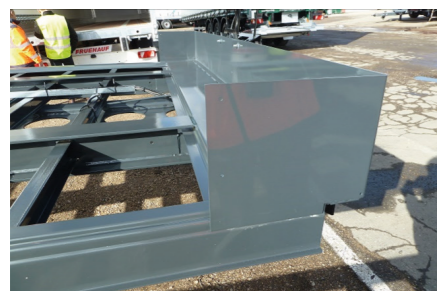
Front protection by steel plinth, welded to the shelf.
