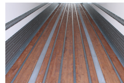
35 mm hardwood laminated floor with steel omega profiles.
