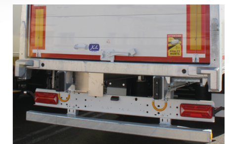
Reinforced rear frame for frequent docking.
