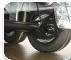
REINFORCED AXLES AND PROTECTED BRAKES
