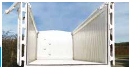
Reinforced modular body with smooth side walls
