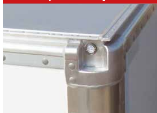
Roof assembly insuring impact resistance and perfect water tightness
