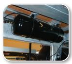
The roller shutter door **EASY**<sup>UP</sup> can be used without any truck. The additional air tank allows more cycles than usually needed between 2 operation of uncoupling and coupling.
